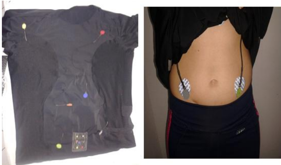
Figure1. T-shirt with Vital Jacket and its electrodes in patient.
